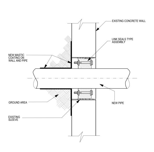
WHERE NEW LINK SEALS CANNOT BE INSTALLED IN EXISTING OPENING PROVIDE A GROUP OF EPDM RUBBER GASKETS EQUIVALENT TO LINK SEAL IN THICKNESS.
