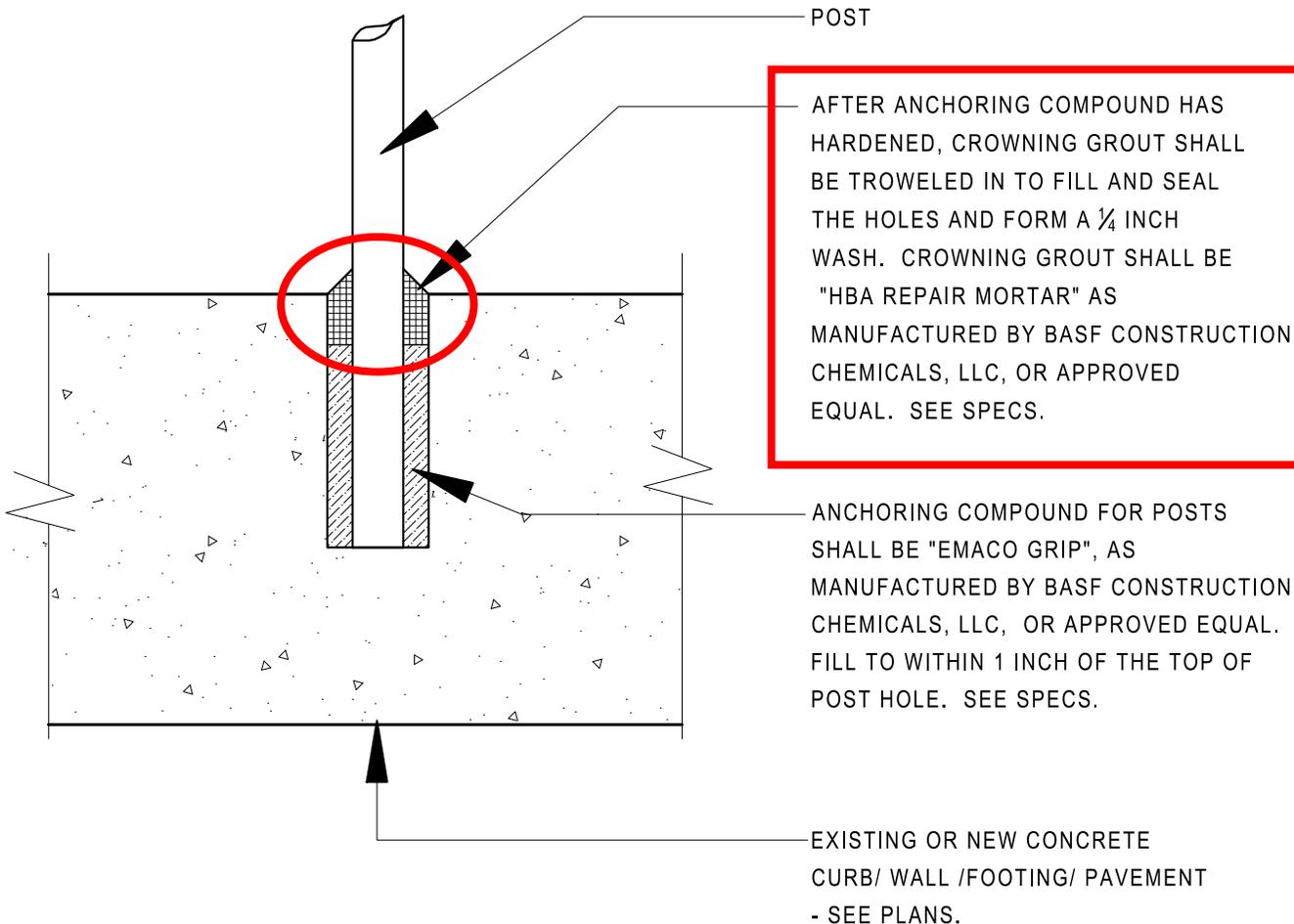
AFTER ANCHORING COMPOUND HAS HARDENED, CROWNING GROUT SHALL BE TROWELED IN TO FILL AND SEAL THE HOLES AND FORM A ¼ INCH WASH. CROWNING GROUT SHALL BE "HBA REPAIR MORTAR" AS MANUFACTURED BY BASF CONSTRUCTION CHEMICALS, LLC, OR APPROVED EQUAL. SEE SPECS.
