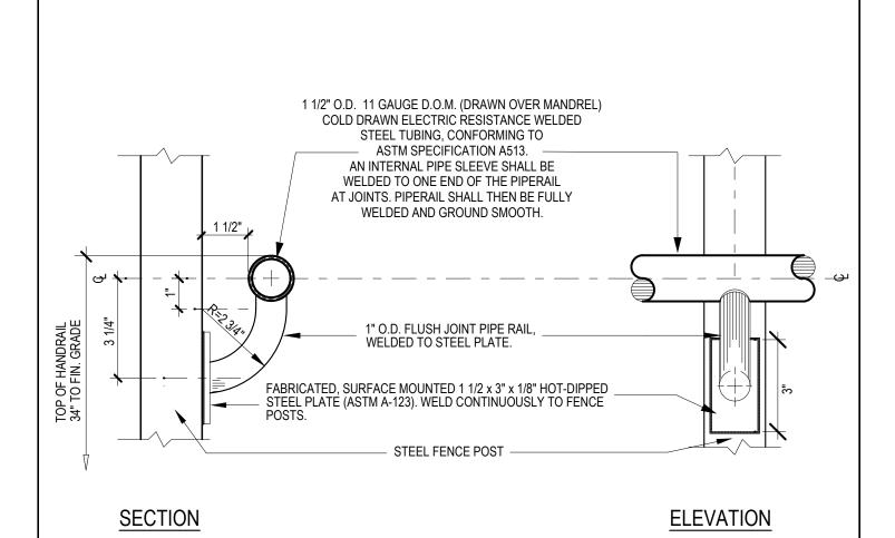
NOTE-PIPE HANDRAIL SHALL BE PAINTED AS PER SPECS. BRACKET SHALL BE WELDED TO ALL SBF POSTS (5' O.C. MAX). FENCE POSTS SHALL BE INSTALLED AT ALL LOCATIONS TO ENSURE PROPER MOUNTING OF HANDRAIL.
