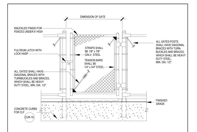
GATES SHALL BE FRAMED ON FOUR SIDES WITH 2 INCH DIA. STANDARD WEIGHT STEEL PIPE. THE GATE FRAMES SHALL BE OF ALL SHOP WELDED CONSTRUCTION WITH COMPLETE FULL WELDS GROUND SMOOTH. THEY SHALL BE THOROUGHLY CLEANED AND HOT DIPPED GALVANIZED IN ACCORD WITH A.S.T.M. SPECIFICATION A-123 AFTER FABRICATION.
