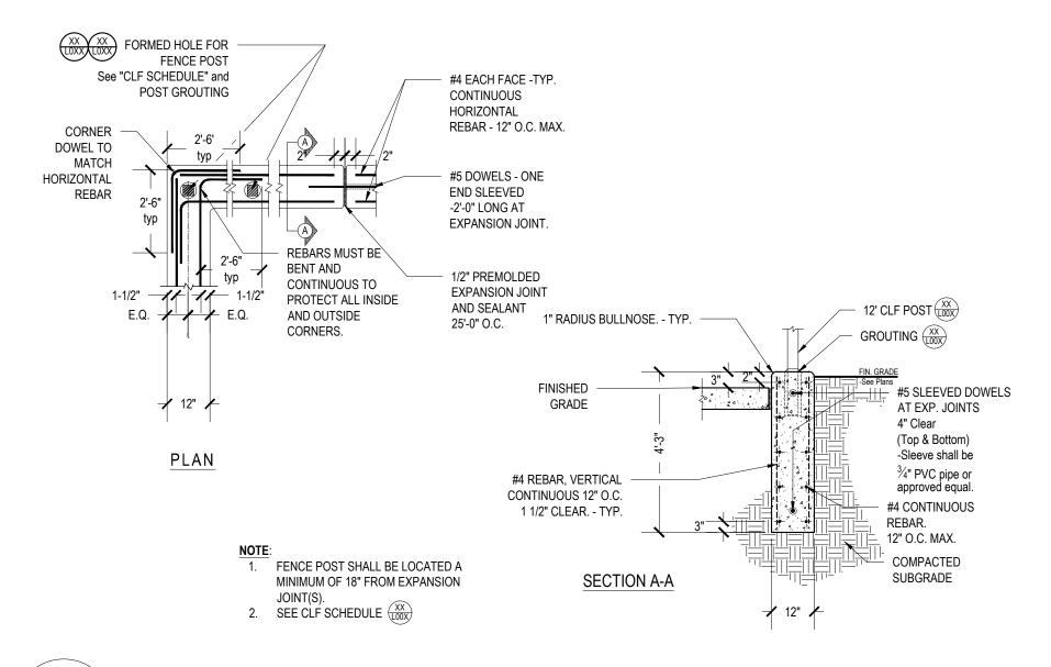
Concrete Curb for 12' Chain Link Fence
