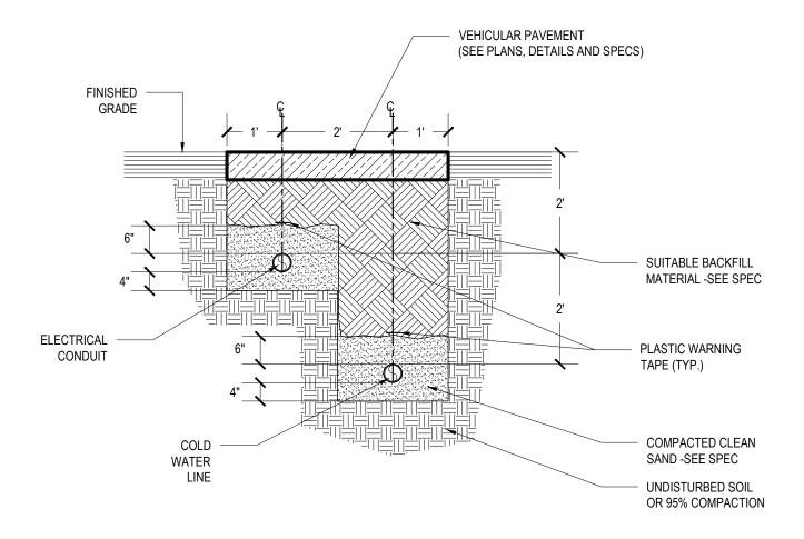
TRENCHING DETAIL FOR ELECTRICAL CONDUIT AND WATER SUPPLY LINE AT VEHICULAR AREA
