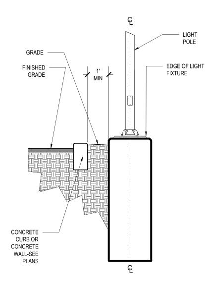
NOTE: THE CONTRACTOR SHALL FIELD VERIFY THE WIDTH OF EXISTING CURB/WALL ELEMENTS TO ALLOW SUFFICIENT ROOM FOR INSTALLATION OF LIGHT POLE FOUNDATIONS.
