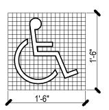
THE ACCESSIBILITY SYMBOL SHALL BE PAINTED ON THE PAVEMENT OF THE PARKING STALL AS SPECIFIED ON THE PLANS AND IN ACCORDANCE WITH THE "AMERICAN NATIONAL STANDARDS INSTITUTE". COLOR SHALL BE BLUE. SEE ASPHALT SPECIFICATIONS.
