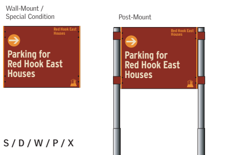
SIGN TYPE B2.1 (Panel - 25" W x 20" H) Parking Directional - Small - Recommended for low-rise developments
