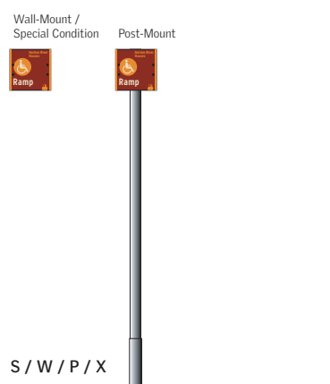
S / W / P / X SIGN TYPE C1.4 (Panel - 7.5" W x 7.5" H) Regulatory Marker - Site-Specific
