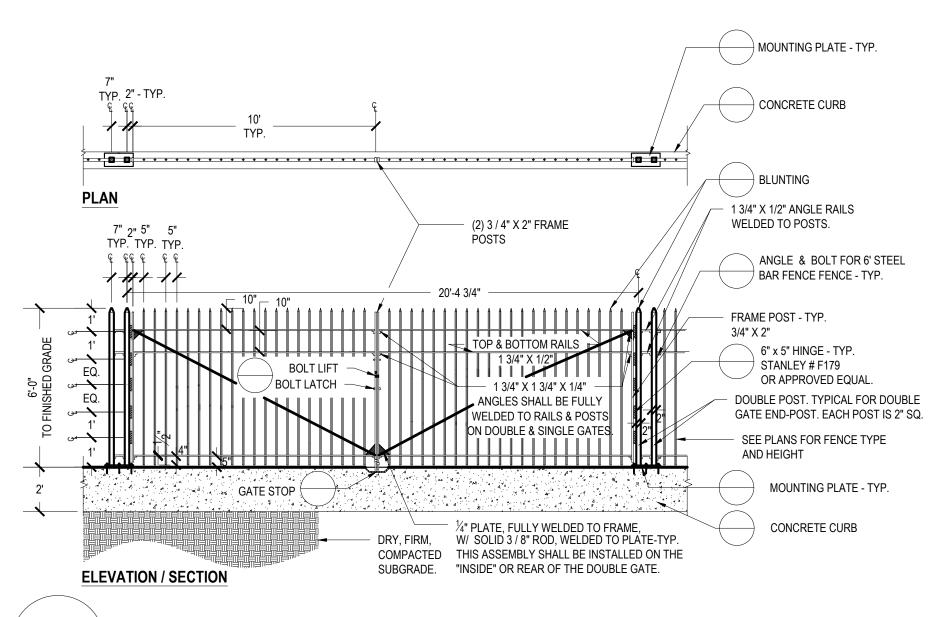
6'-0" STEEL BAR FENCE WIDE DOUBLE GATE IN FLUSH CONCRETE CURB FOR COMPACTOR AREAS
