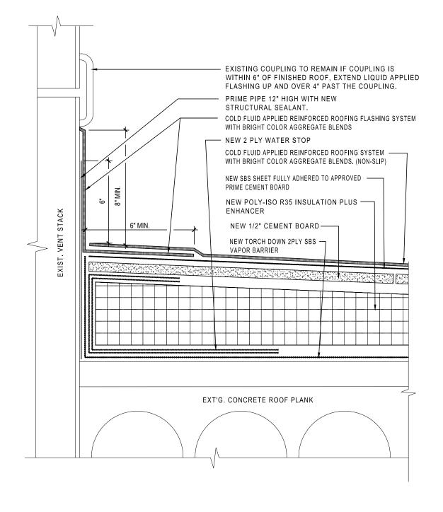
3 FLASHING DET. @ STACK VENT
