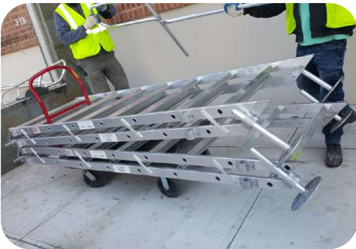
Deployable stairs on a hand cart in Oceanside cannot be bolted to the ground.
